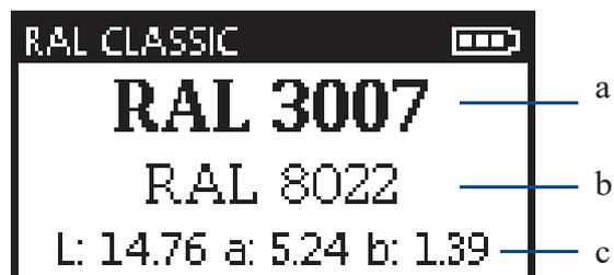
Figure 5. Display with a measurement result
