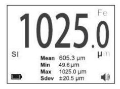
If the measurement is outside the alarm limits, the unit will beep three times to signal this.
