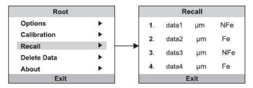
To clear the data, press Then move to the menu item "Data deletion" via the main menu for the options menu. Then you can choose DATA between "single deletion" (deletion of individual data) and "total deletion" (deletion of all values).
