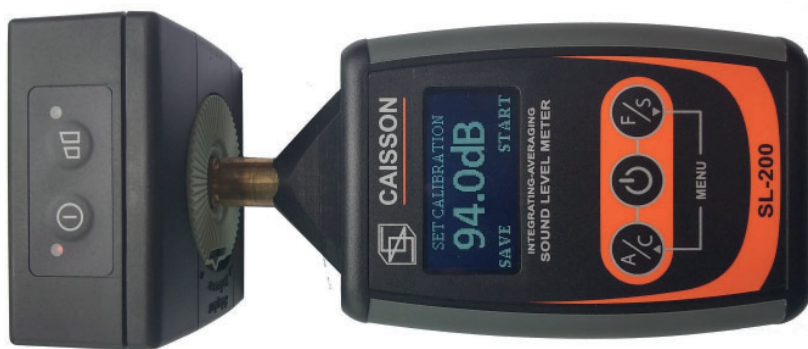
Fig. 3.1 Sound Level Calibrator fitted onto your sound level meter
