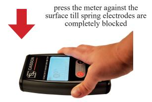
It is recommended to repeat the measurement in a few points situated next to each other as humidity has a tendency of uneven distribution. If the measurements vary, only the highest outcomes should be used.
